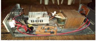
Fig.2: The Picture of the Assembled 0.75kVA Inverter 5. Results and Discussions
